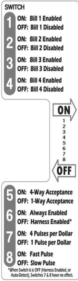
**Configuration using the DIP Switches**
